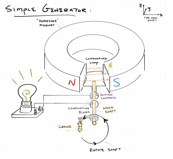
Turning crank rotates wire loop between magnet poles, inducing an emf which is used to power a light bulb.
