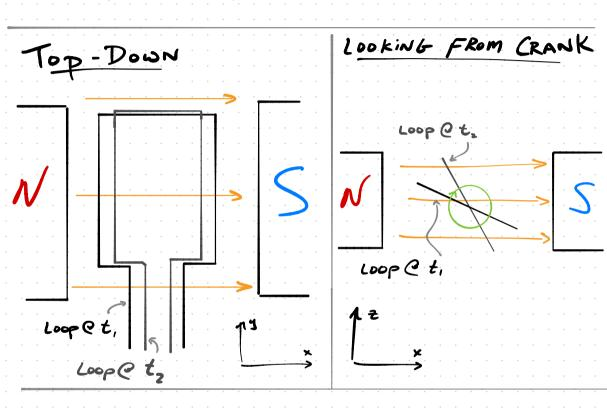
What is the emf generated in loop as it rotates at a constant rate? · CONSTANT ROTATION:
