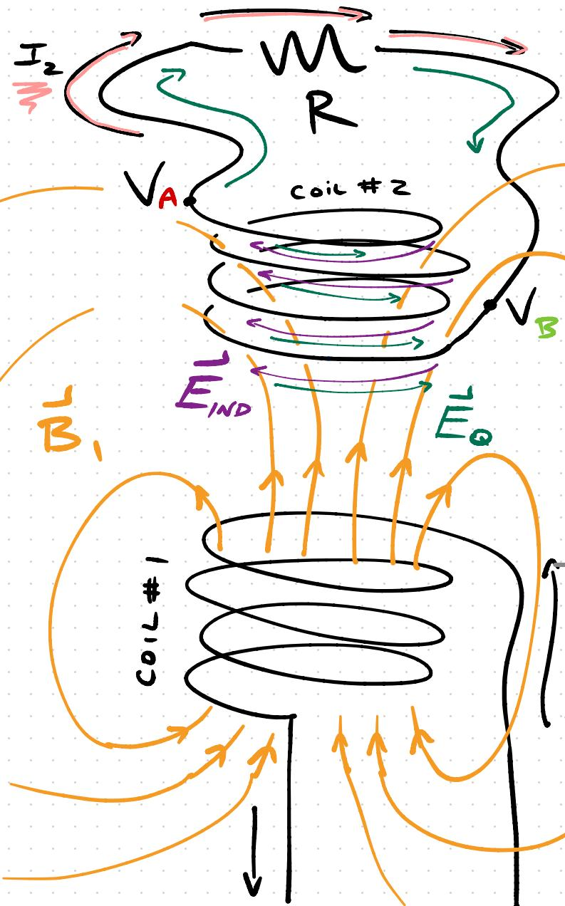
But now there is a voltage drop  $V_A - V_B = \text{EMF}$  across the resistor, causing a current  $I_2 = \frac{\text{EMF}}{R}$
