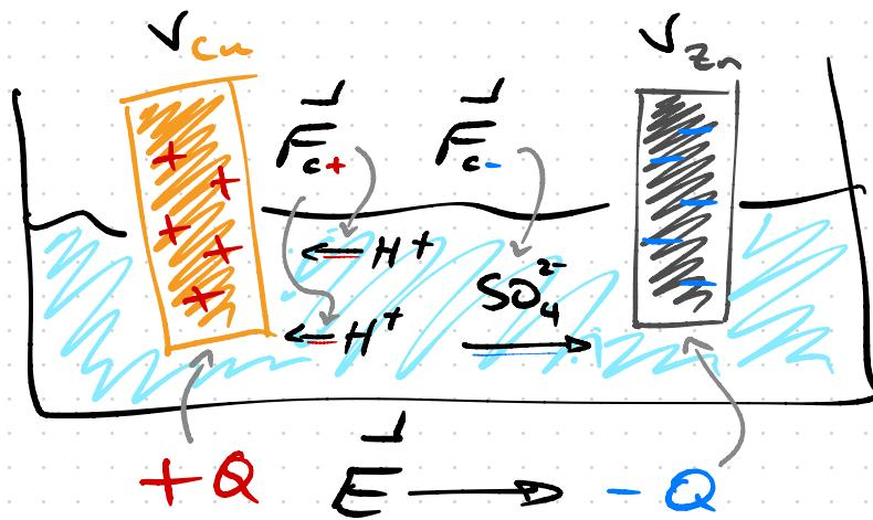
$$@ V_{Cu} - V_{Zn} = \text{EMF} :$$
