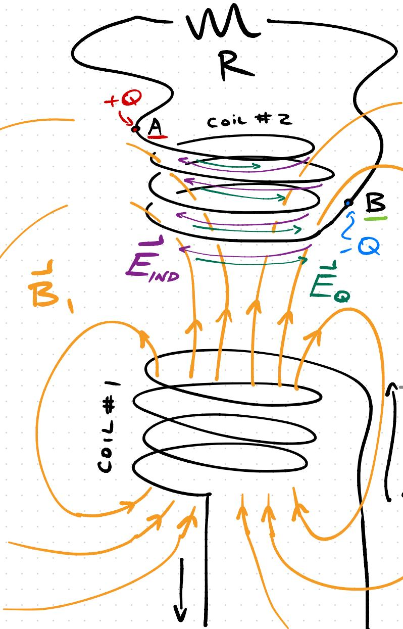
WHEN  $E_{IND}$  HAS TRANSFERRED ENOUGH CHARGE  $+ Q$  SO THAT  $V_A - V_B = \text{EMF}$ , THEN  $E_{IND}$  IS CANCELLED BY  $E_Q$  FROM  $+ Q$ .
