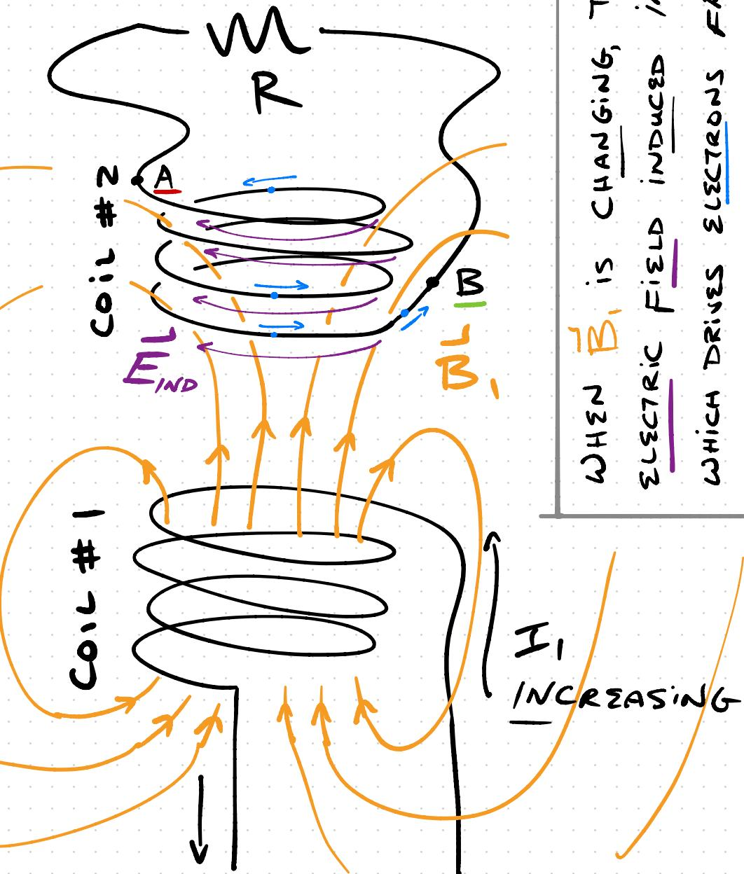
WHEN  $B_i$  is CHANGING, THERE IS AN ELECTRIC FIELD induced in COIL #2, WHICH DRIVES ELECTRONS FROM ONE END OF COIL (A) TO OTHER (B).
