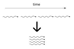
If we take, say, 1 Joule of energy, which is the amount of energy your hand absorbs by pointing it at the sun for 1 second, and compress it all into 10 ns =  $10 \times 10^{-9}$  s, then we obtain  $P = \frac{E}{\Delta t} = 100$  MW in power. We can further increase the proximity of the photons in our pulse if we also *focus* the light with a lens:
