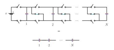
We are now finished rearranging our connections and we find we have taken our N capacitors that were originally connected in parallel and connected them in series. To determine the voltage V that across this series connection we make a couple observations:
