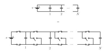
The actual circuit is the lower diagram. If we take note of which switches are open and which are closed, we find it is electrically equivalent to the upper diagram<sup>2</sup>. Since the capacitors are connected in parallel, the voltage across all of them is the same (why?). By inspecting the diagram we see that they are connected to the positive and negative end of the voltage source, so that the voltage across the capacitors is v. Therefore the charge  $\pm Q$  on each capacitor is
