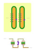
In the updated schematic we have eliminated the discharged capacitor<sup>4</sup>. What we end up with is electrically equivalent to the final configuration of the Marx bank; that is, we obtain a series connection of capacitors with opposite charges. The potential difference between the two ends of a stack of electrocytes is therefore the *sum* of the membrane potentials of all the electrocytes in the stack.
