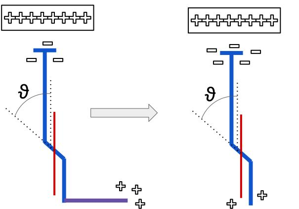
Answer: Charge separation induced by charged object results in negative charge on the electroscope and positive charge on the grounding bar. Removing the bar leaves the negative charge on the electroscope.
