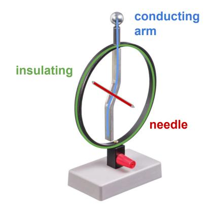
Device for detecting the presence and polarity ( + or - ) of electric charge.
