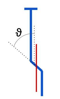
The electroscope (conducting arm + needle) is initially uncharged.
