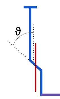
Same scenario as previously, but now we have electrically connected the bottom of the electroscope to a **long "grounding" bar**, pointing away from the positively charged object.
