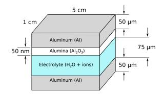
Assuming the sheets are perfectly flat, what is the capacitance of this capacitor? Pick the answer closest to your calculated result:
